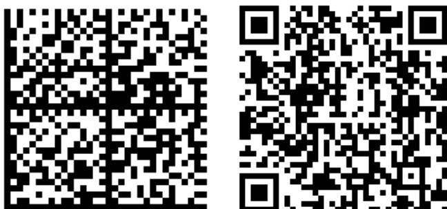
Figure 1. Data Matrix (left) and QR code (right) with coded text: IS'11 Automatic identification based on 2D barcodes
