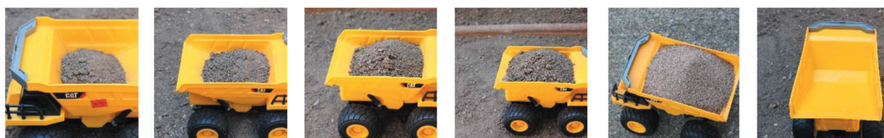
Figure 2. Images of dump trucks for 200ml, 400ml, 600ml, 800ml, 1000ml, and empty loads
