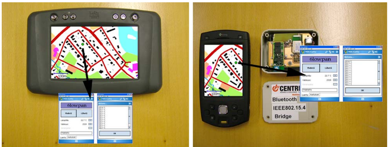
Figure 5. In-situ monitoring with mobile devices in Locawe platform. Left: directly over 6LoWPAN communication with a handheld device; Right: over a Bluetooth bridge (LM-048 module from LM Technologies and RadioCraft's RC2301AT module).
